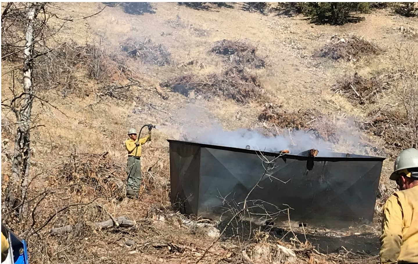
Quenching the kiln once a full load has been converted to biochar
